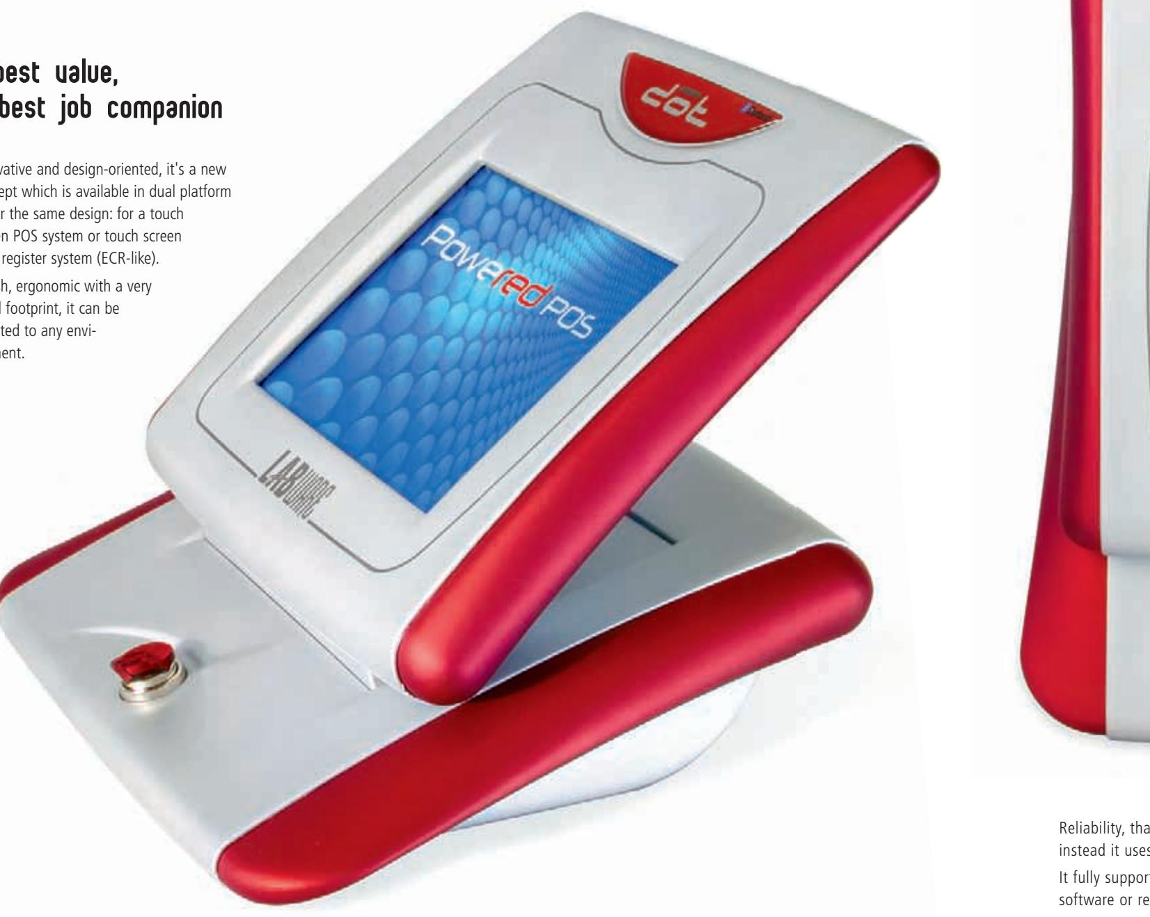
Reliability, that makes your life relaxed, is guaranteed by the firmware solution design. It has no hard drive, instead it uses on board flash memory and with the total absence of any fan it is an extremely robust system. It fully supports any POS peripherals, such as kitchen printers, scanners, scales and connects to a back office software or remote PC for polling and program maintenance.
